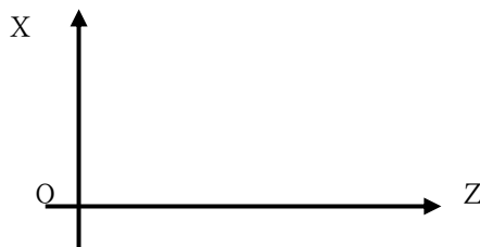
Fig. 1-2 X-Z plane rectangular coordinate system 2 (rear tool post coordinate system)
